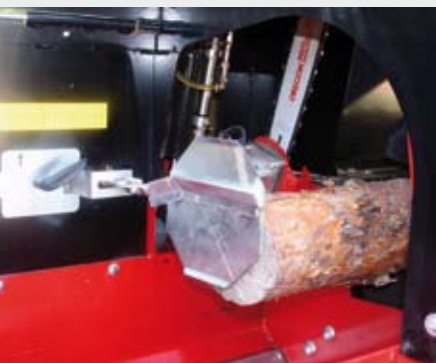
EXPERT and PRO models equipped with a hydraulic log stopper (BASIC models with mechanic).
