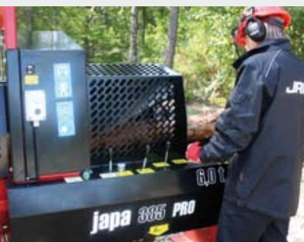
New hydraulic safety mechanism stops splitting and sawing when the hydraulic splitting cover is open.
