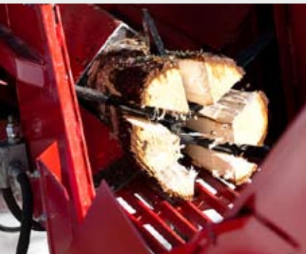
6-way knife available as optional (in PRO models as standard).
