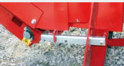
The unloading conveyor can be easily turned to 3 different positions, 20° to the left and right.
