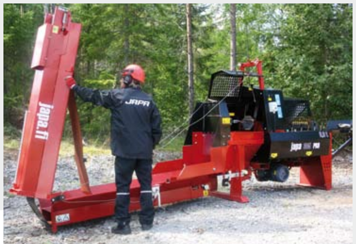
Unloading conveyer with a central joint can be easily set into operating position, using a winch.
